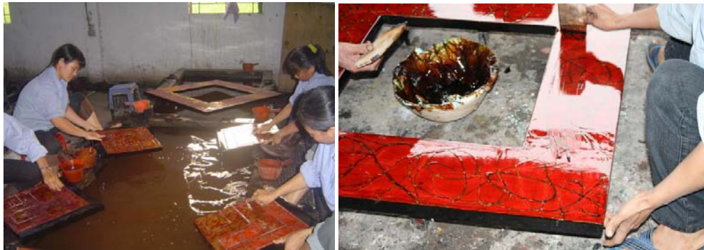
Figure 8. Water scarping/grinding (left) and shiny painting (right)
